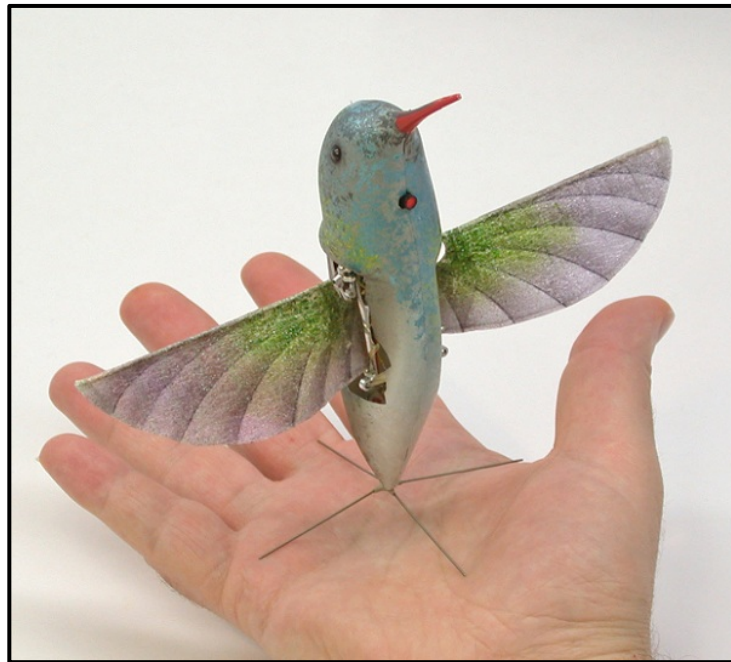
Figure 2.2: This UAV can record video and audio while being controlled by an operator. The UAV is designed to convince any objects of surveillance that there is no video or audio recording of their conduct. This particular model is an example of the rapid development and increased sophistication of UAV function and designs. The UAV is no longer just an eight-foot drone with a camera lurking obtrusively in the air. Now, UAVs can take on new forms and functions and with that, new operations.
