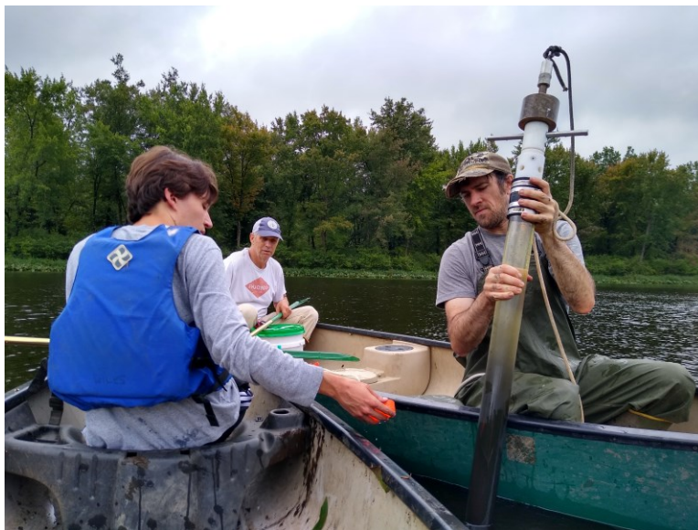
Fig. 25. Sampling Brown's Lake's sediment-water interface with a probing instrument.
