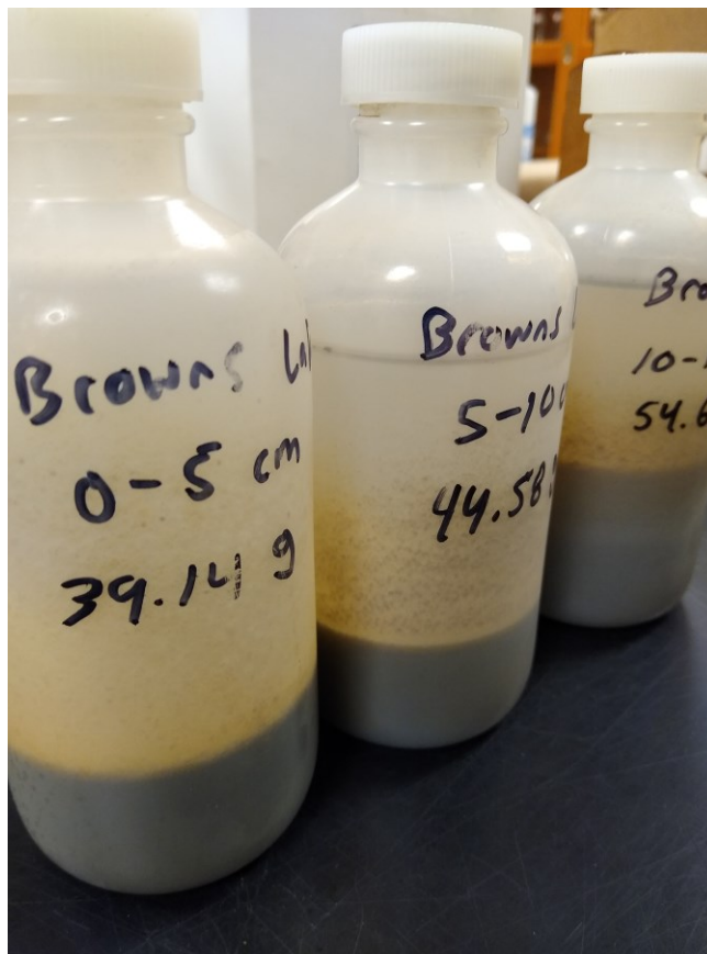
Fig. 27. Sediment suspension after settling for at least a day.
