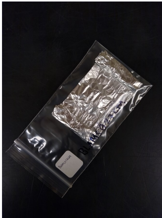
Fig. 26. Peat-filled sediment wrapped in aluminum foil for AMS radiocarbon dating.
