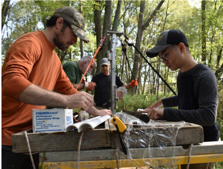
Fig. 24. Describing sediment cores on-site. The modified-Livingstone corer is in the background.
