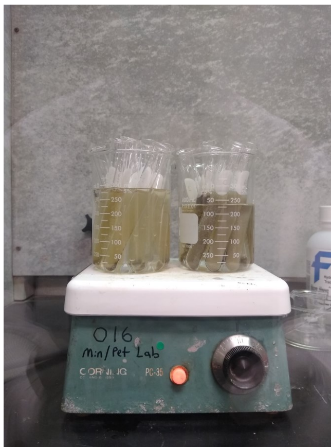
Fig. 28. Oxidizing organics with hot hydrogen peroxide.
