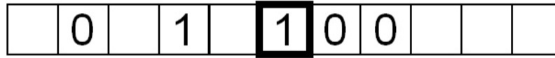
Figure 5.1: A representation of the tape of a Turing machine. The location of the head of the machine is bold [17]
