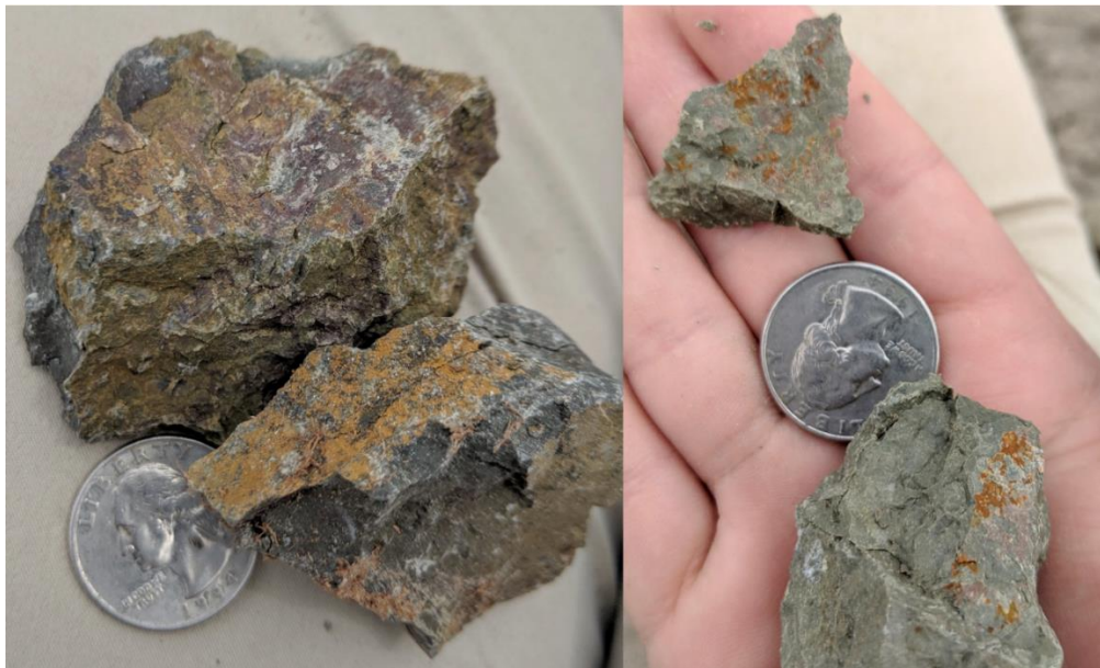
Figure 10. Observing hand samples from stratigraphic section CORY 19-58 to determine grain size, matrix color, mottling color, and mottling percent.
