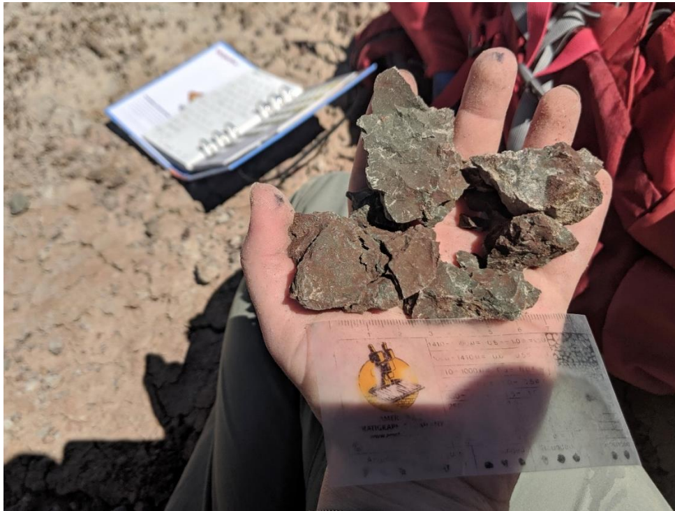
Figure 10. Observing hand samples from stratigraphic section CORY 19-58 to determine grain size, matrix color, mottling color, and mottling percent.
