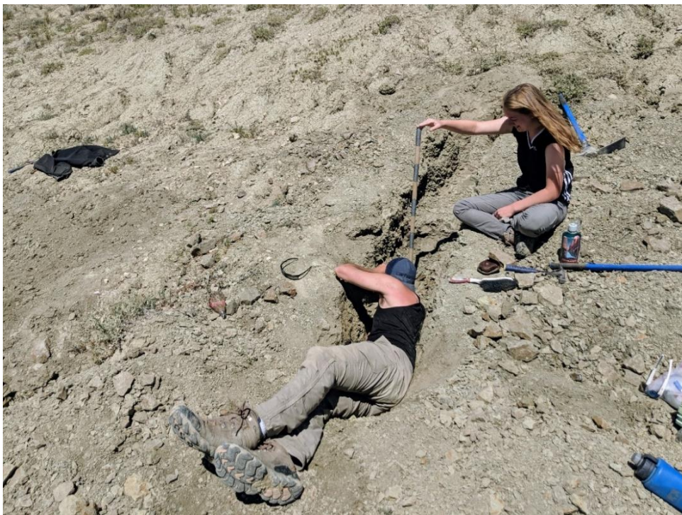
Figure 9. Measuring units in stratigraphic section CORY 19-35 using a Jacob's staff.
