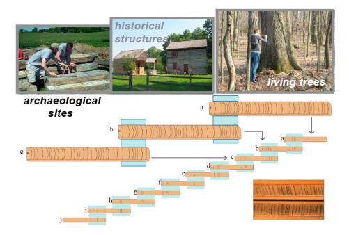
**Figure 1.** Diagram illustrating tree-ring cross-dating. Patterns in ring widths from archaeological and historic structures are compared to living tree ring chronologies in order to assign calendar dates to each ring.
